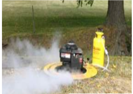
Figure 9: Smoke Testing Blower
